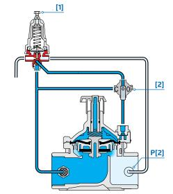
The Pressure Reducing Pilot [1] commands the main Valve to throttle closed should Downstream Pressure [P2] rise above pilot setting, and to open fully when it drops below pilot setting. The Manual Selector [2] enables local manual closing.
