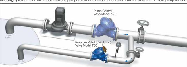
The Model 730 relieves over pressure caused by excessive pump discharge during low demand. To keep a constant discharge pressure, the difference between pumped flow and consumer demand can be circulated back to pump suction.
