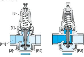
The Upstream Pressure [P1] applies balanced opening and closing hydraulic forces under the Diaphragm [1] and above the Plug [2]. Downstream Pressure [P2] applies hydraulic closing force under the plug, which seeks to reach equilibrium with the Set Spring [3] force. Should [P2] rise above setting, the hydraulic closing forces rise above the mechanical force of the spring, pushing the plug to modulate closed, and reducing [P2] back to setting.
