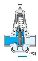
The Upstream Pressure [P1] applies balanced opening and closing hydraulic forces under the Diaphragm [1] and above the Plug [2]. Downstream Pressure [P2] applies hydraulic closing force under the plug, which seeks to reach equilibrium with the Set Spring [3] force. Should [P2] rise above setting, the hydraulic closing forces rise above the mechanical force of the spring, pushing the plug to modulate closed, and reducing [P2] back to setting.
