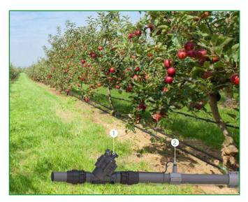
BERMAD Model IR-100-LMOe opens when the system reaches closure pressure flushing dirt and sediment out, and shuts off upon line pressure build-up when irrigation begins.
