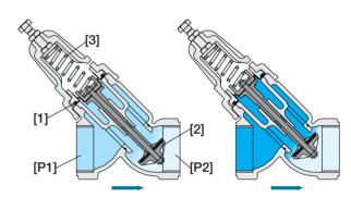
The Upstream Pressure [P1] applies balanced opening and closing hydraulic forces under the Diaphragm [1] and above the Plug [2]. Downstream Pressure [P2] applies hydraulic closing force under the plug, which seeks to reach equilibrium with the Set Spring [3] force. Should [P2] rise above setting, the hydraulic closing forces rise above the mechanical force of the spring, pushing the plug to modulate closed, reducing [P2] back to setting, and eventually shutting drip-tight.
