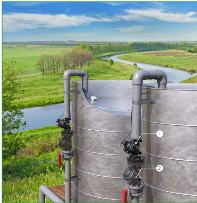
[1] BERMAD Model IR-150-60 opens upon drop in reservoir level maintaining "Always Full" reservoir, and shuts on rise in reservoir level to preset high.
