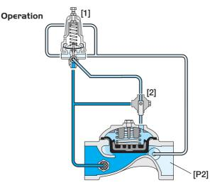
The Pressure Reducing Servo Pilot [1] commands the main Valve to throttle closed preventing downstream pressure [P2] from rising above pilot setting, and to modulate open when [P2] drops below pilot setting. The Manual selector [2] enables local manual closing.
