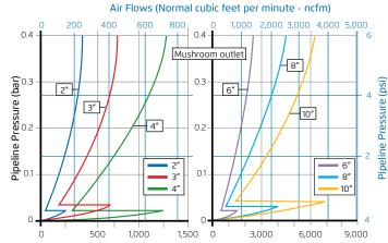
Air Flow (normal cubic meter per hour - nm<sup>3</sup>/h)
