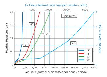
Air Release (Pressurized Operation)
