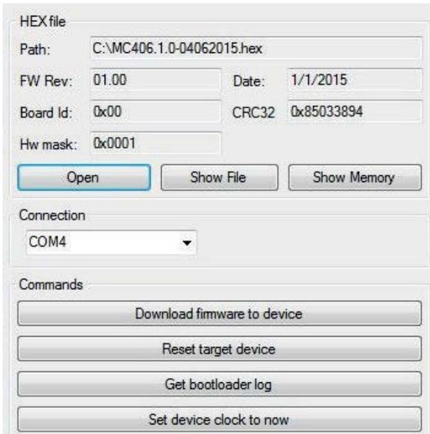
After selecting the firmware file and the proper COM port the converter must enter in boot mode; this can be done by cycling the power or by pressing the “Reset target device” button; the LCD will show the bootloader CRC32 and version.
