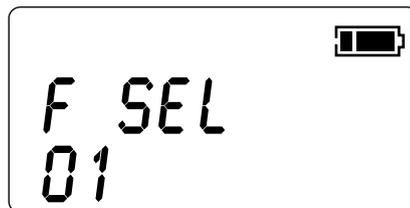
function selection code: every value corresponds to a parameter set menu or function (see 11. FUNCTIONS); to select the function code use P4 / P3; to enter the selected code use P2. Pressing P1 returns to the main screen
