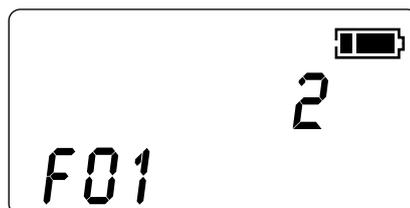
inside a specific function, the pushbuttons functionality may differ (see 11. FUNCTIONS); in this example, P4 / P3 increase and decreases the parameter value shown on the first row, P2 confirms the value and move back to the function selection, P1 abort the operation and goes back to the main screen.
