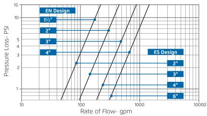
Cv=Valve flow coefficient (flow in gpm at  $\Delta P=1$  psi) Q=Flow rate (gpm)  $\Delta P=$ Differential pressure (psi)
