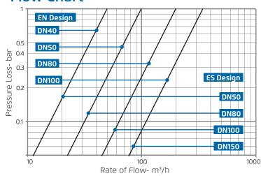
Kv=Valve flow coefficient (flow in m<sup>3</sup>/h at  $\Delta$ P=1bar) Q=Flow rate (m<sup>3</sup>/h)  $\Delta$ P=Differential pressure (bar)
