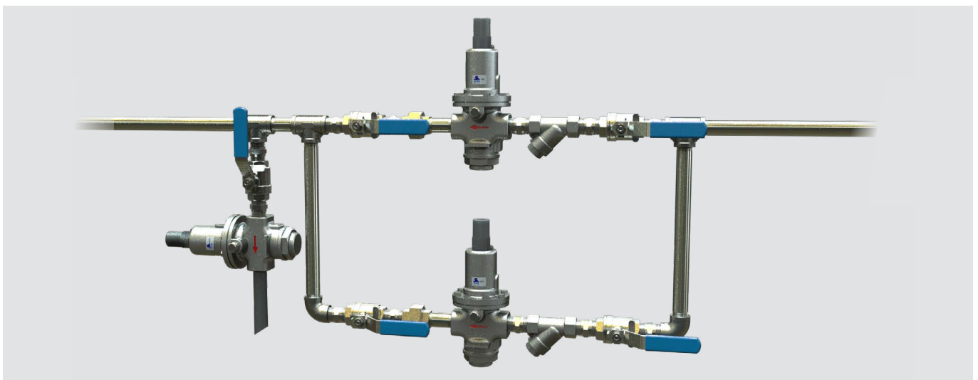
Pressure reducing system with redundancy for small pressure zones featuring BERMAD DPRV-#2HC direct acting pressure reducing valve and BERMAD DPRV-#3HC direct acting pressure relief valve.
