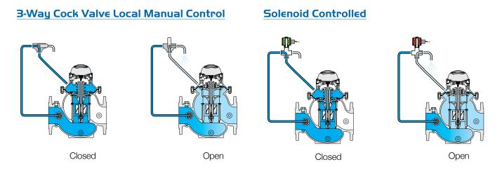
Line pressure is applied to the control chamber of the hydrometer through the opened 3-way solenoid or cock valve. This creates superior hydraulic force in the control chamber that causes the valve to close and seal drip tight.
