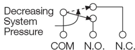
Typical Low Pressure Supervision
