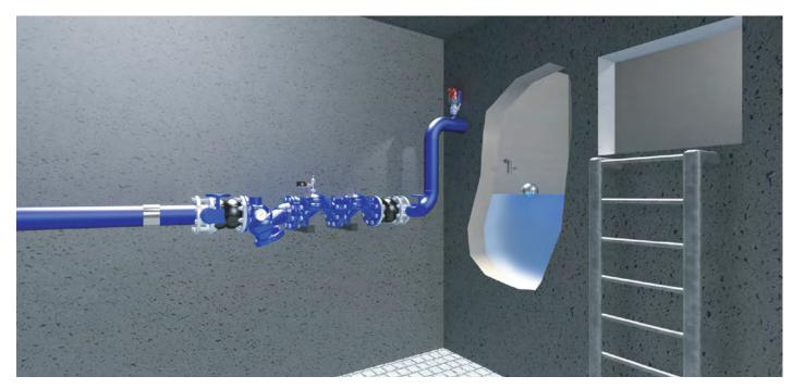
Water Reservoir Level Control System, featuring the 450-60 that maintains constant water level in the reservoir. As backup another level control valve is stationed upstream and calibrated to a slightly
