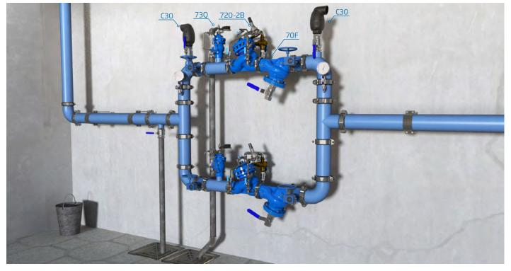
Pressure Reducing Station, featuring BERMAD 720-2B valves to reduce high incoming pressure to a lower downstream set-point, a redundant, parallel branch to minimize the possibility of total water shut-off. The embedded low flow by-pass saves on installation of
