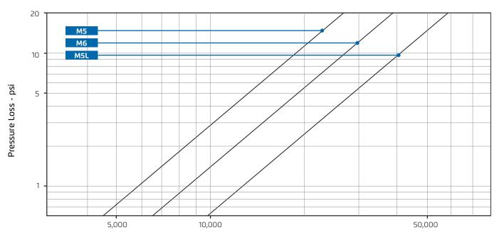
Flow Rate - gpm (Water)
