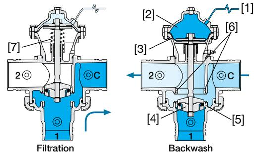
A Hydraulic Command [1], which pressurizes the Upper Control Chamber [2], forces the Diaphragm [3] actuated Plug Assembly [4] to move towards the Supply Port Seat [5], eventually sealing it drip tight. This allows flow from the filter through the Drain Port Seat [6]. Venting the upper control chamber causes the line pressure, together with the Spring [7] force, to move the Valve back to filtration mode.
