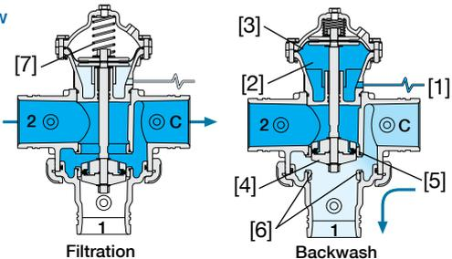
A Hydraulic Command [1], which pressurizes the Lower Control Chamber [2], forces the Diaphragm [3] actuated Plug Assembly [4] to move towards the Supply Port Seat [5], eventually sealing it drip tight. This allows flow from the filter through the Drain Port Seat [6]. Venting the upper control chamber causes the line pressure, together with the Spring [7] force, to move the Valve back to filtration mode.
