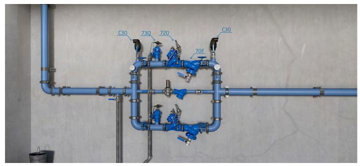
Pressure Reducing Station, featuring BERMAD 73Q valves to relieve excessive downstream pressure, a redundant, parallel branch to minimize the possibility of total water shut-off and a low flow
