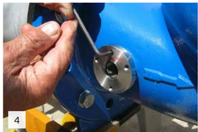
4 Fasten the fixing screw using 4mm Allen key to prevent the disk from twisting
