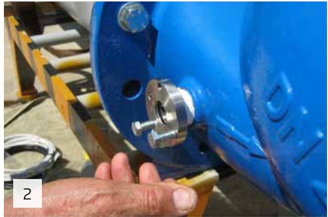
2 Screw the sealing disk into the 1" BSPT port; use two regular screws to lock the disk temporarily in the up-right position as indicated on the disk. Tighten the disk gently
