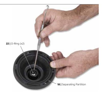
Use a silicon lubricant when reassembling the shaft.
