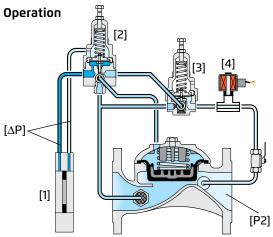
Pressure Differential [ $\Delta P$ ] across the Orifice Assembly [1] is in direct proportion to demand. The Flow Pilot [2] continuously senses [ $\Delta P$ ] and commands the Valve to throttle closed should demand rise above pilot setting, and to modulate open when demand drops. The Pressure Reducing Pilot [3] controls the Valve to prevent Downstream Pressure [P2] from rising above pilot setting. The Solenoid [4] closes in response to an electric signal, shutting the main Valve.
