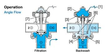
A Hydraulic Command [1], which pressurizes the Upper Control Chamber [2], forces the Diaphragm [3] actuated Plug Assembly [4] to move towards the Supply Port Seat [5], eventually sealing it drip tight. This allows flow from the filter through the Drain Port Seat [6]. Venting the upper control chamber causes the line pressure, together with the Spring [7] force, to move the Valve back to filtration mode.
