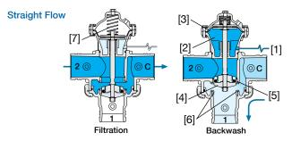
A Hydraulic Command [1], which pressurizes the Lower Control Chamber [2], forces the Diaphragm [3] actuated Plug Assembly [4] to move towards the Supply Port Seat [5], eventually sealing it drip tight. This allows flow from the filter through the Drain Port Seat [6]. Venting the upper control chamber causes the line pressure, together with the Spring [7] force, to move the Valve back to filtration mode.
