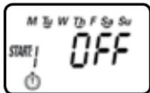
2. Press the
