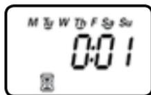
4. If the required irrigation duration is less than an hour press the
