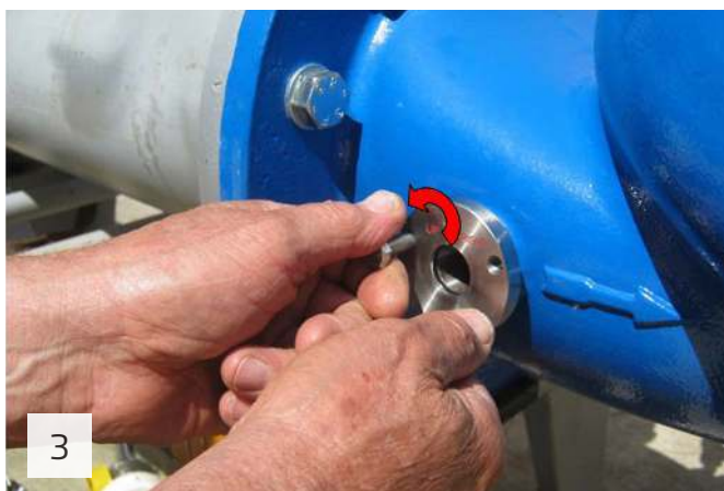
Remove the temporary screws from the disk
