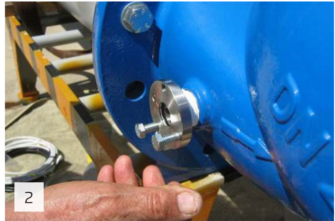
Screw the sealing disk into the 1" BSPT port; use two regular screws to lock the disk temporarily in the up-right position as indicated on the disk. Tighten the disk gently
