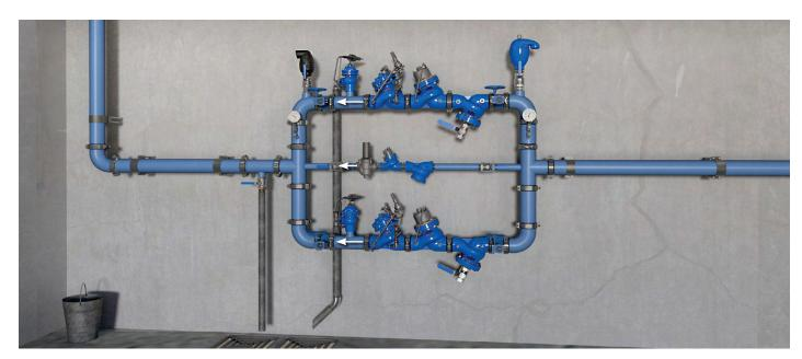
**Pressure Reducing Station**, featuring BERMAD BC-80F-P Strainers to protect each branch from foreign debris, a redundant, parallel branch to minimize the possibility of total water shut-off and a low flow bypass branch for low demand operation. For information on the
