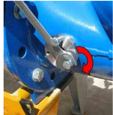
Screw the sealing disk into the 1" BSPT port; use two regular screws to lock the disk temporarily in the up-right position as indicated on the disk. Tighten the disk gently
