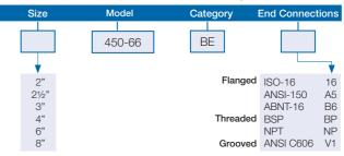
Pressure Rating: 16 bar (230 psi) Valve Pattern: Globe & Angle (2"-4") Working Temperature: Water up to 60°C (140°F) Main Construction Materials: Body, Cover and Actuator: Ductile Iron Internals: Stainless Steel & Elastomer
