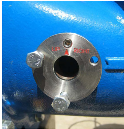
Screw the sealing disk into the 1" BSPT port; use two regular screws to lock the disk temporarily in the up-right position as indicated on the disk. Tighten the disk gently
