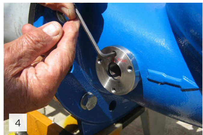
Fasten the fixing screw using 4mm Allen key to prevent the disk from twisting
