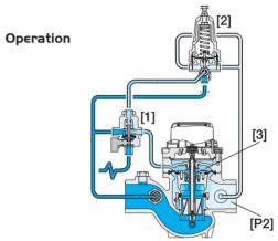
The 3-Way Hydraulic Relay Valve (3W-HRV) [1] hydraulically connects the Pressure Reducing Servo Pilot (PRSP) [2] to the Hydrometer Control Chamber [3]. The PRSP commands the Hydrometer to throttle closed, preventing Downstream Pressure [P2] from rising above pilot setting. The 3W-HRV switches upon pressure drop command, directing line pressure into the control chamber, and thereby causing the Hydrometer to shut. The 3W-HRV also features local manual closing.
