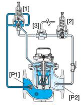
The Pressure Sustaining pilot **[1]** commands the Hydrometer to throttle closed should Upstream Pressure **[P1]** drop below pilot setting, and modulate open when **[P1]** rises above it. When **[P1]** is high, the Pressure Reducing Pilot **[2]** commands the Hydrometer to prevent Downstream Pressure **[P2]** from rising above pilot setting. The Hydraulic Relay Valve **[3]** closes upon pressure rise command, shutting the Hydrometer.
