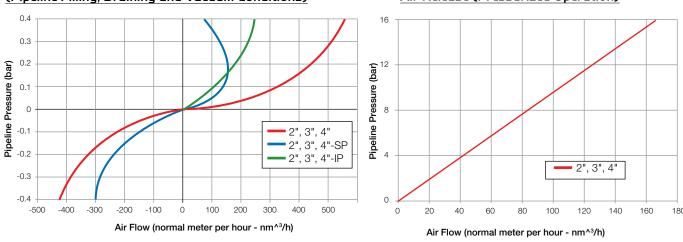
Air relief and intake charts are based on actual measurements, made during 2015 in Bermad Air Flow test bench, according to EN-1074/4 standard and refer to Side outlet.
