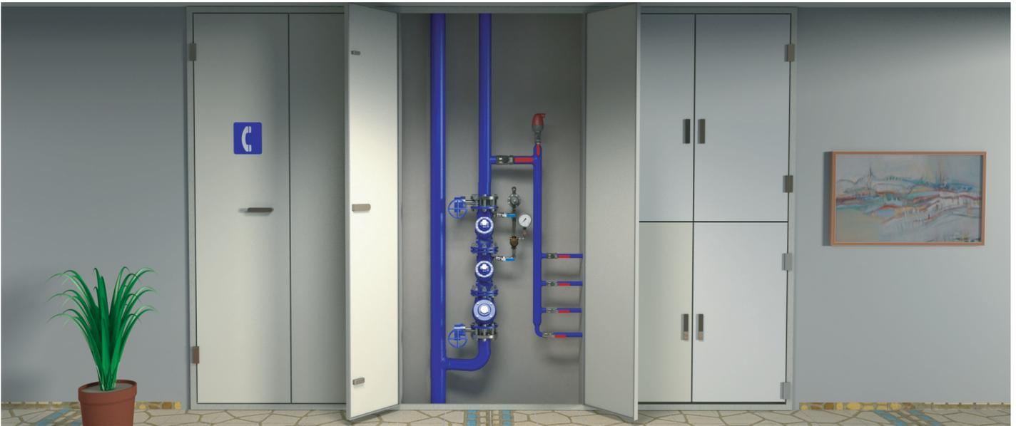
**Pressure Reducing System**, featuring a BERMAD BC-72S-B2H-P system to reduce high incoming pressure to a lower downstream set-point while minimizing the possibility of total water shut-off, a low flow bypass for
