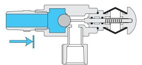
**Closed:** When the system piping suddenly fills with water/fluid the drip check closes.
