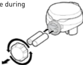
**Attention: note for the proper polarity direction as marked on the bottom of the controller's housing.**
