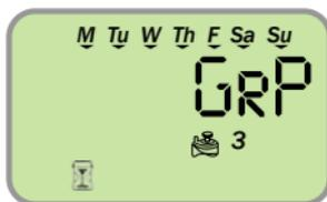
**For example: the above screen shot shows that valve number 3 operates together with valve 2 and according to the irrigation program of valve 2.**
