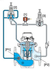
Opening the Solenoid [1] opens the Hydrometer, which continuously transmits flow data to the irrigation controller. The Pressure Sustaining pilot [2] commands the Hydrometer to throttle closed should Upstream Pressure [P1] drop below pilot setting, and to modulate open when [P1] rises above it. When [P1] is high, the Pressure Reducing Pilot [3] commands the Hydrometer to prevent Downstream Pressure [P2] from rising above pilot setting. Closing the solenoid causes the Hydrometer to shut.
