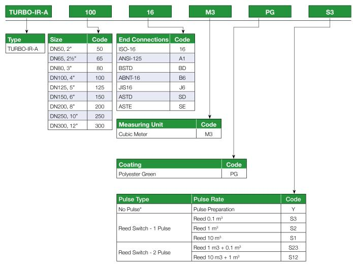
\* When ordering "No Pulse" (Pulse Preparation) write "Y" & the possible future Pulse Rate Example: Turbo-IR-A-3"-16-PG-M3-Y/S3
