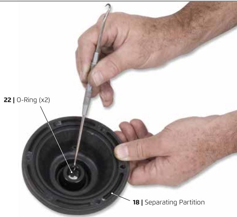
Use a silicon lubricant when reassembling the shaft.
