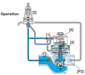
The Shut-Off Pilot (SOP) [1] connects the Pressure Reducing Pilot (PRP) [2] to the AMV Control Chamber [3]. The PRP commands the AMV to throttle closed should Downstream Pressure [P2] rise above setting and to open fully when it drops below setting. Upon delivering the preset quantity of water, the AMV manually preset Control Head Mechanism [4] switches the SOP, which directs line pressure into the control chamber causing the AMV to shut.
