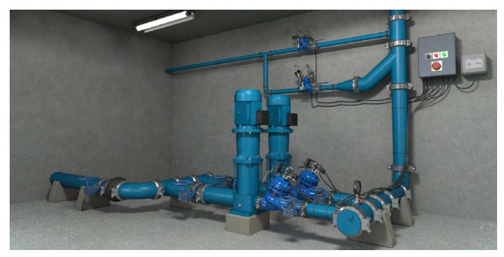
**Pump Station**, featuring the BERMAD BC-740-P valves to slowly introduce pump pressure to the system or slowly remove pump pressure from the system in response to a signal from the pump controller. In power failure situations,
