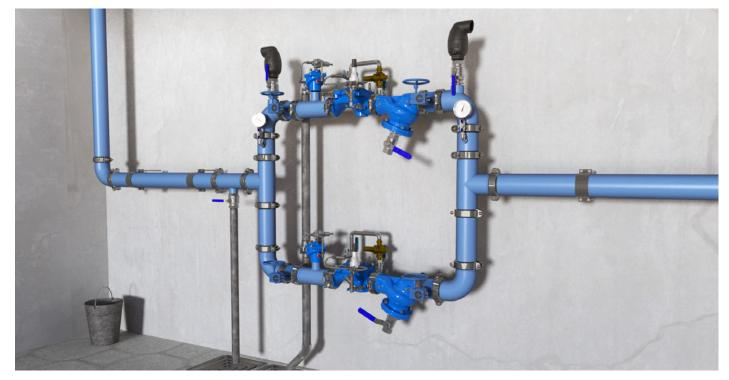
Pressure Reducing Station, featuring BERMAD BC-420-2B-P valves to reduce high incoming pressure to a lower downstream set-point, a redundant, parallel branch to minimize the possibility of total water shut-off. The imbedded low flow by-pass saves on installation of
