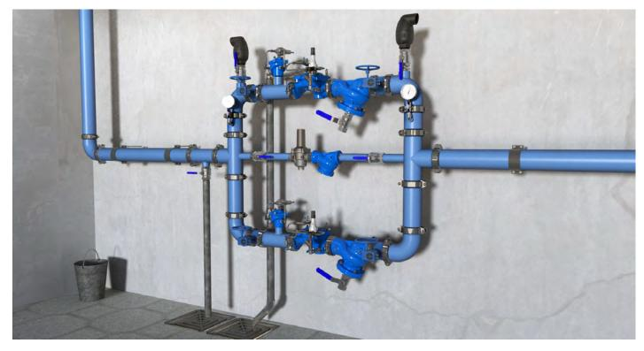
Pressure Reducing Station, featuring BERMAD BC-420-P valves to reduce high incoming pressure to a lower downstream set-point, a redundant, parallel branch to minimize the possibility of total water shut-off and
