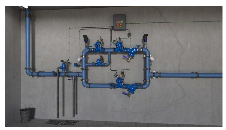
Pressure Reducing Station with Block Valve and Automatic Backup. In case of abnormal pressure rise detected by the PS the system switches automatically between the active branch and the backup branch and an indication is sent to the BMS.
