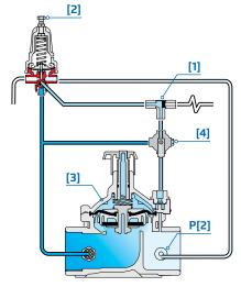
The Shuttle Valve [1] hydraulically connects the Pressure Reducing Pilot (PRP) [2] to the Valve Control Chamber [3]. The PRP commands the Valve to throttle closed should Downstream Pressure [P2] rise above setting and to open fully when it drops below setting. Upon pressure rise command, the shuttle valve automatically switches, allowing pressurization of the control chamber, which causes the main Valve to shut. The Manual Selector [4] enables manual closing.
