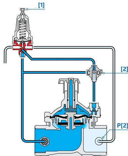
The Pressure Reducing Pilot [1] commands the main Valve to throttle closed should Downstream Pressure [P2] rise above pilot setting, and to open fully when it drops below pilot setting. The Manual Selector [2] enables local manual closing.
