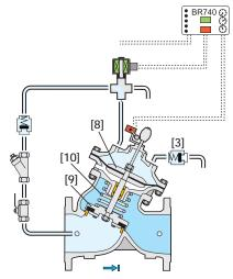
Closed (After Power Failure)
