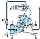
The Pressure Relief pilot [1] commands the Valve to open immediately should the upstream pressure [P1] abruptly rise above pilot setting, and to close smoothly when it falls below pilot setting. The Vented Cock Valve [2] enables manual operating test.
