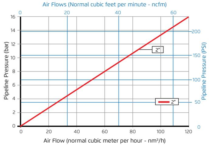
Air relief and intake charts are based on actual measurements, made in Bermad Air Flow test bench, according to EN-1074/4 standard and refer to Side outlet.
